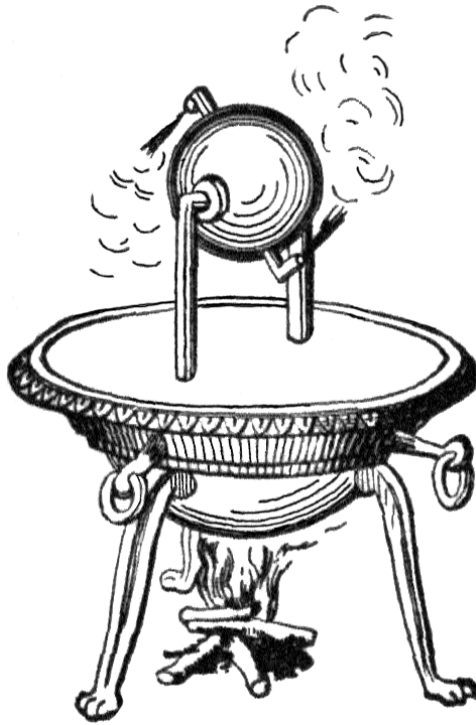
Author unknown. Aeolipile illustration . 1876. Bron: Wikimedia Commons.
